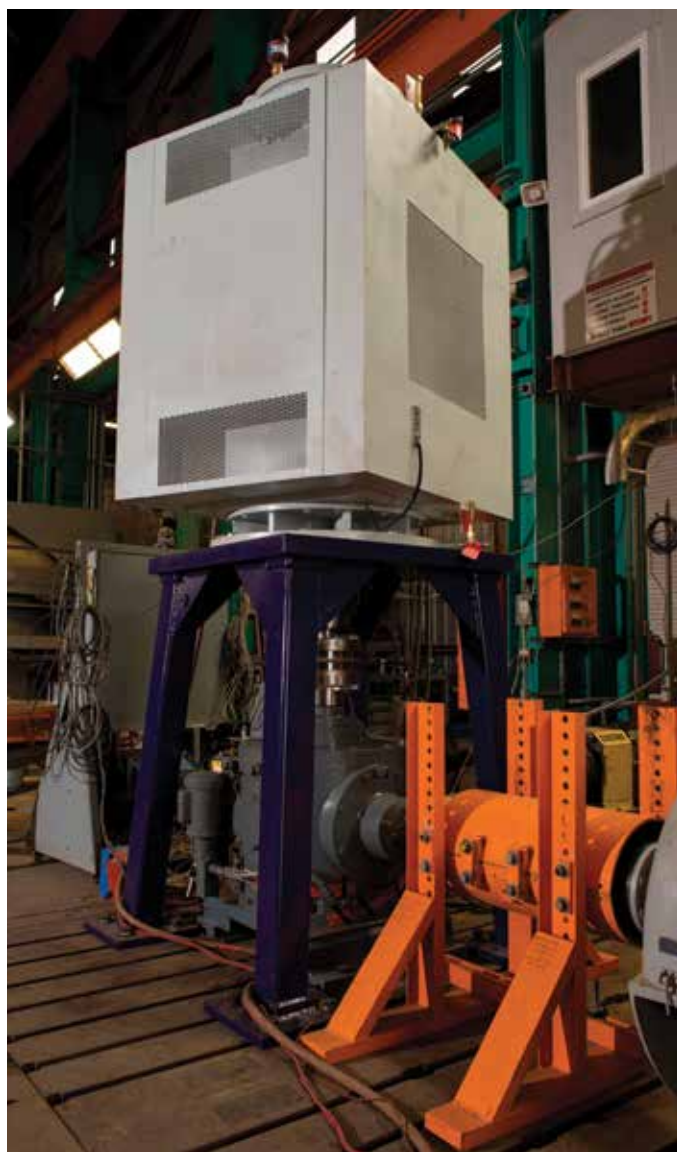
Bradleys, Inc. load tests a 1,750 horsepower, 1,800 RPM, 4,000 Volts, vertical motor.
